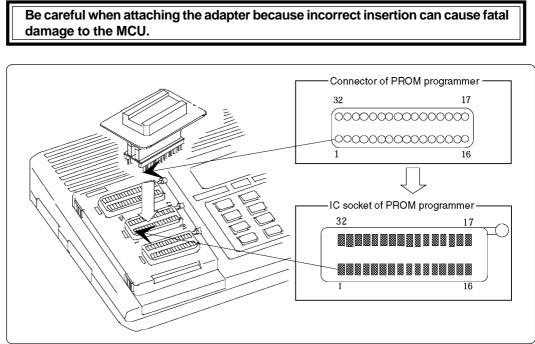
Figure 3.1 Attaching the adapter to a PROM programmer
